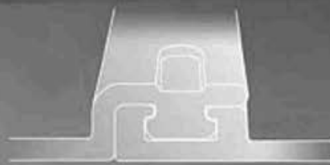
Joining by stamping (gives visible deformations)
